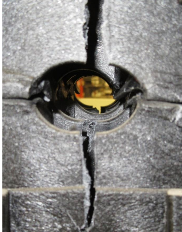
Figure 6. Splitting of the interior utility holes after testing of Specimen 2.
