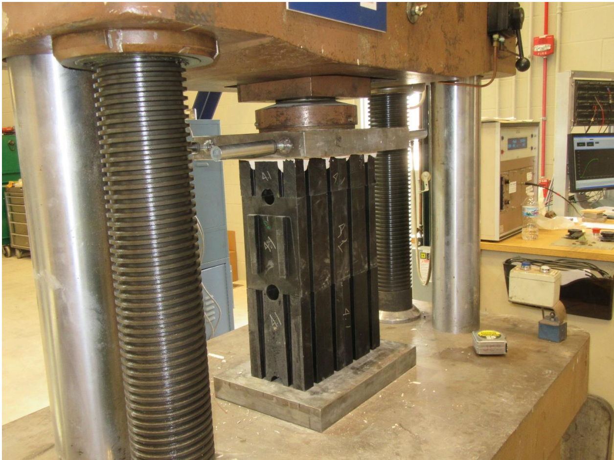
Figure 3. A typical test specimen in the load frame.
