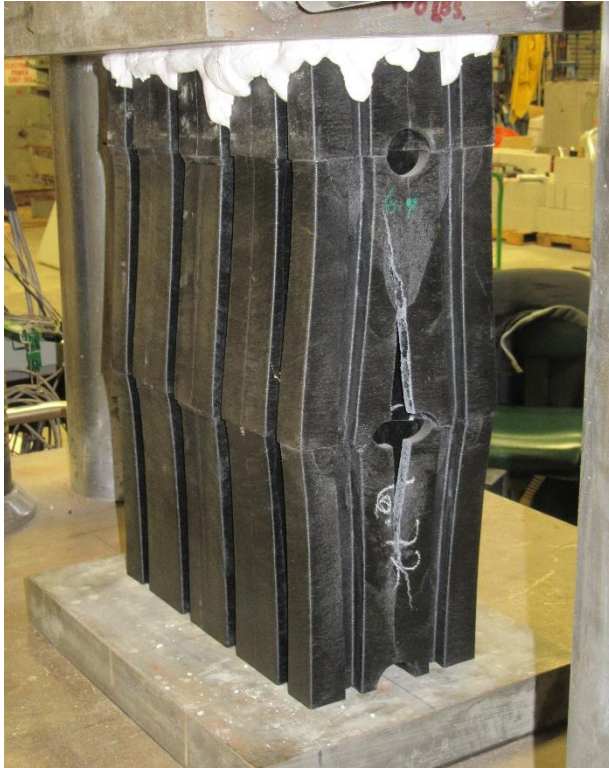
Figure 7. Tensile splitting and local crushing of Specimen 2 during testing.
