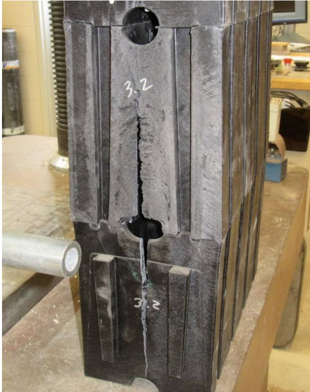
Figure 5. Splitting tensile failure around the lower utility hole in Specimen 8.
